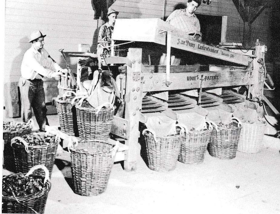
Fig. 14. Bulb grading is also done with the help of machinery. (Photo courtesy of Lee Merrill, Tacoma, Washington.)
